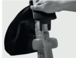
Insert the adjustable handle to into the leaf blower body adjust the handle to suitable yourself,tighten knob screw(until the handle fully fasten).
